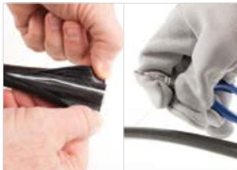
Pull the string to the desired exposure length. Cut off outerjacket with a utility knife (taking care not to cut into the underlying cable jackets).
