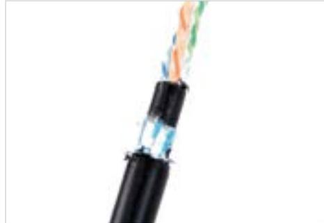
To expose the pairs, cut the inner jacket circumferentially at the intended end of the inner jacket and slide the jacket off the cable end, taking care not to damage the cable pairs.
